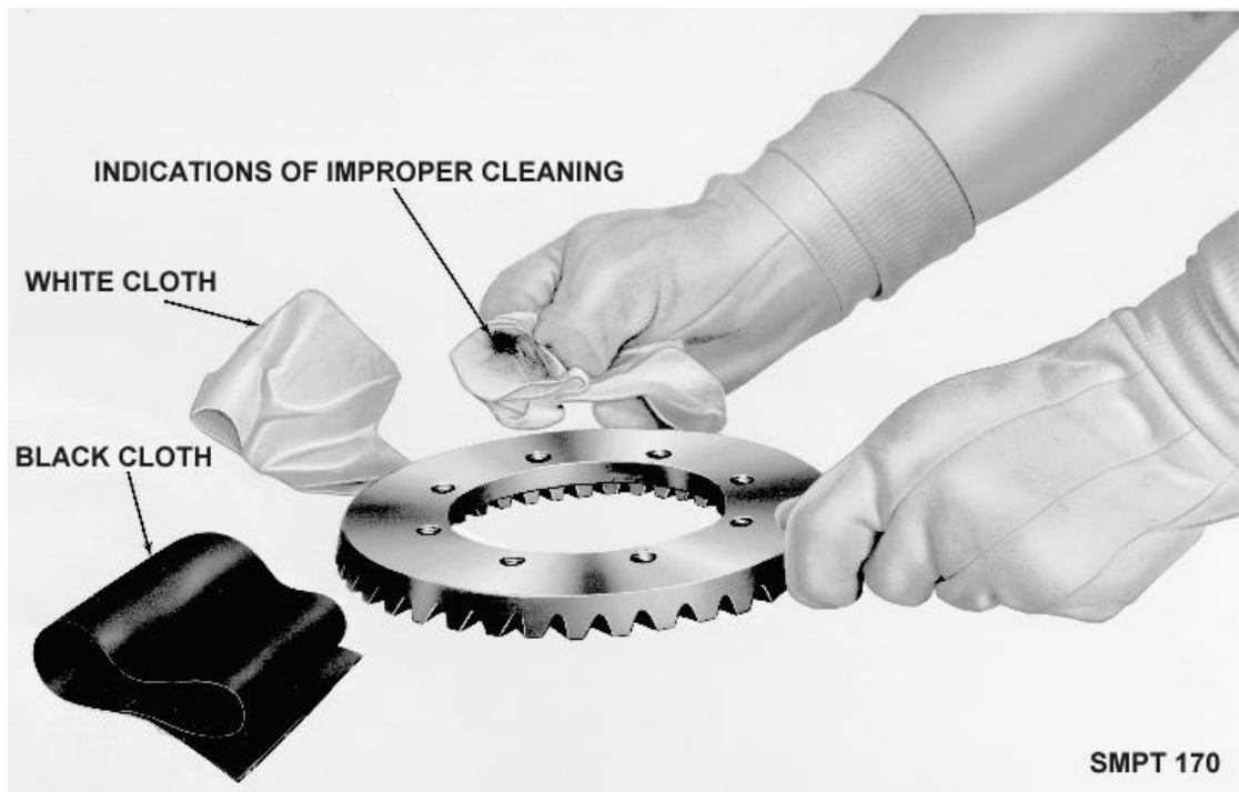
Figure 2-39. Wipe test for cleanliness.
