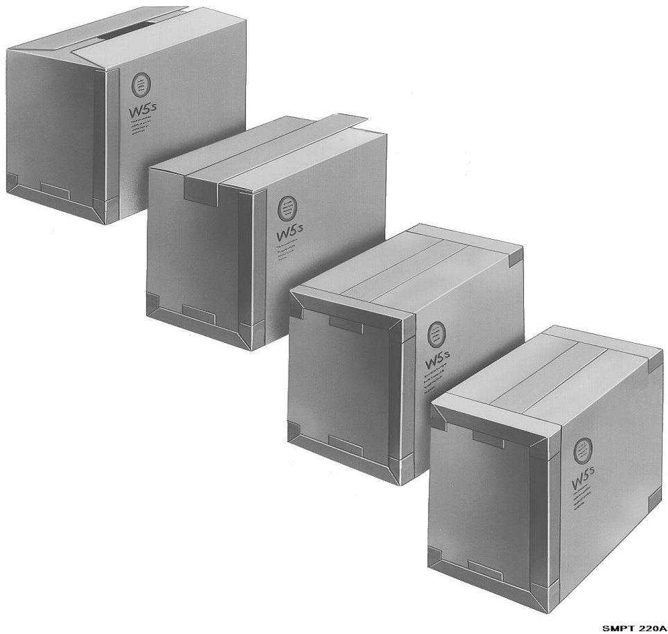
Figure 6-12. Waterproofing fiberboard boxes with tape.
